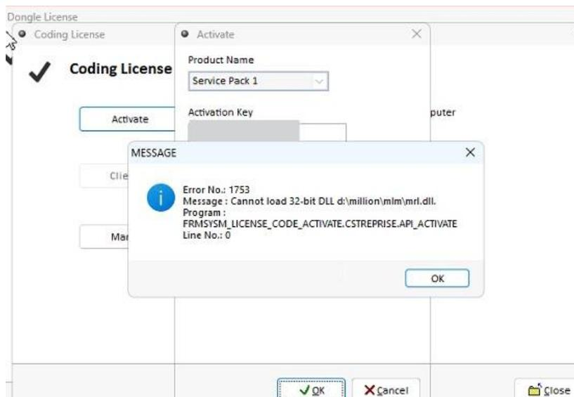
Showing the message “Error No: 1753 Cannot load 32-bit DLL” when activating the Service Pack License.
